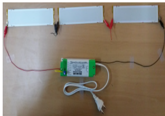
Connection Method (Flexible Type Panels)
